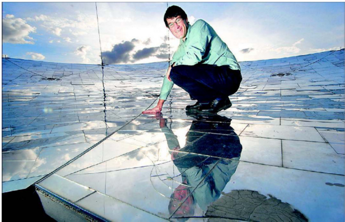
SILVER LINING: Dr Keith Lovegrove, of the ANU College of Engineering and Computer Science, checks the large silver dish that concentrates the sun's rays into a chemical reactor. Picture: BRAHAM TIDY
