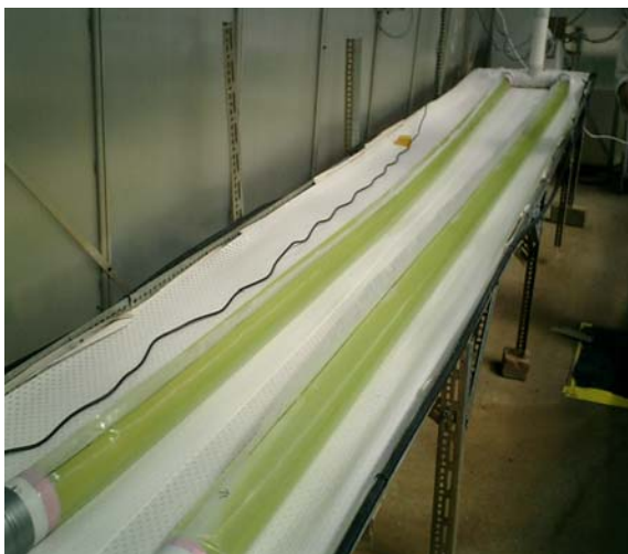
Figure 6. A 50 L, 8 m long photobioreactor prototype in a greenhouse, inoculated with C. reinhardtii .
