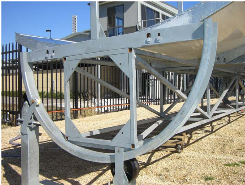
Figure 2.4 View of box frame, hoops and roller wheels
